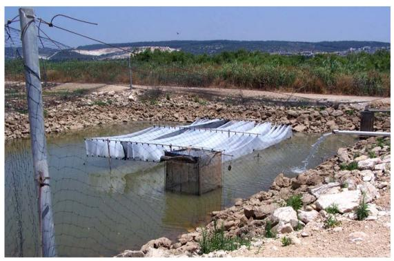
Figure 1: Experimental systems; substrates for periphyton growth in the tilapia culture experiments and the cage in which the substrate experiments were performed; picture taken before the pond was completely filled with water.
